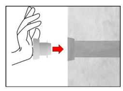
1. Insert the plug into the hole in the concrete wall easily by hand.
