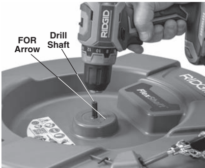
Figure 4 – Attaching Drill To Drill Shaft
