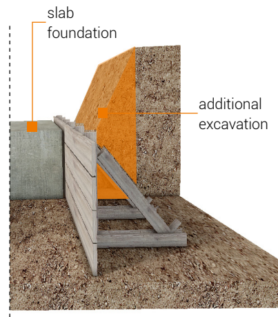
excavation - traditional formwork
