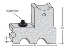
The mounting Bipo oD with nailing sleeve is a fibre-concrete spacer which is used for vertical and horizontal reinforcement. The nailing sleeve is placed into the spacer on factory side and works as a dampener of the force, while hammering in the nail. This reduces the risk of breakage of the spacers. On the construction site, the spacer is attached to the formwork with a stainless steel nail, which guarantees a fast and trouble-free installation of the reinforcement.
